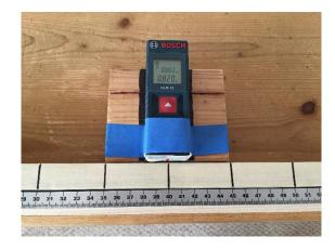
Participants should now slide the laser device every 5 cm and then take and record their readings on their data recording sheet. In the center column, they record the readings as they are on the device display (i.e., in millimeters). In the next column, they round off to the nearest centimeter.
