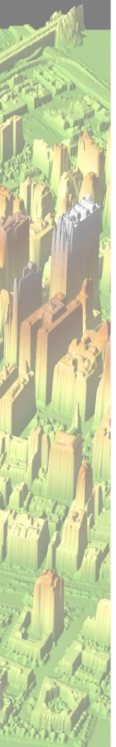
Lidar measurements are often made by airplanes flying over a landscape. The laser sweeps back and forth, and computers use all of the data gathered to piece together a map of the ground beneath. Trigonometry must be used to account for the fact that lidar sweeps back and forth at an angle and not always straight down.
