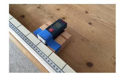
Notice that the block and laser device slide against the reference track.
