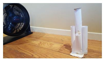
Have participants place their tower (with metal washer on top) about 10 feet away from the fan and then move it closer a little at a time until it is affected by the wind. For each tower, record the distance between the base of the fan and the front edge of the tower. See who can design the tower that can stand still closest to the fan.
